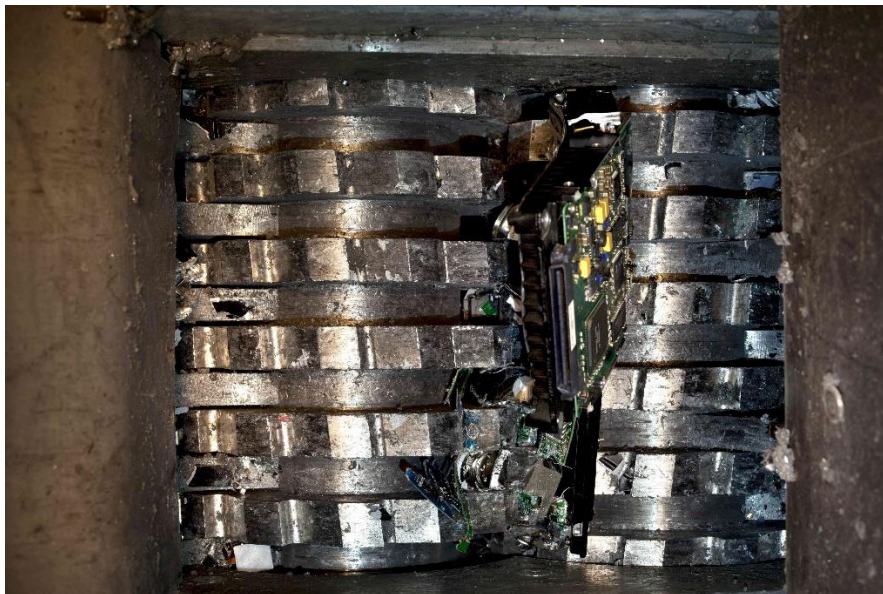
Figure 7: Shredding of e-scrap
